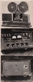
Smaller size "Carfied Sound" 16mm. recorder, middle, amplifier with anti-ground-noise and compressor circuit, bottom, portable power supply.
